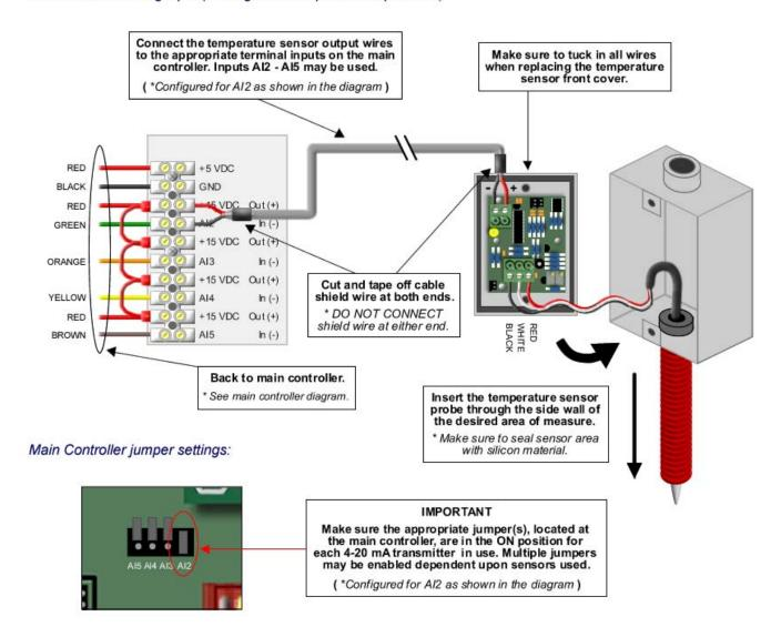
Use 18AWG twisted, stranded, and shielded 3 conductor wire for all sensor connections.
